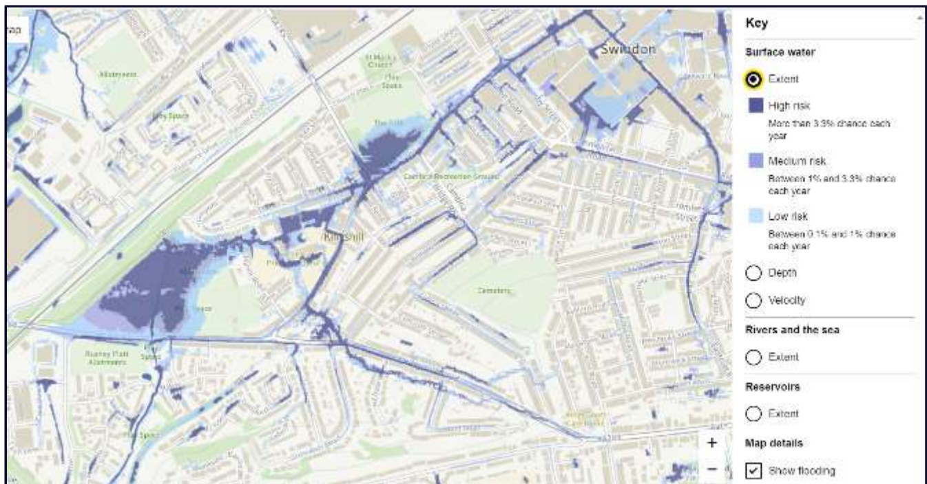
Figure 5 Environment Agency Surface Water Flood Map for Central Swindon
